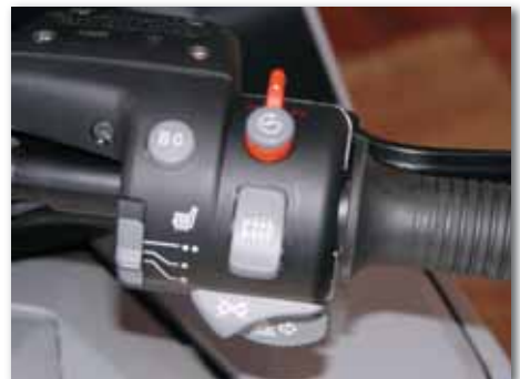
Right-hand controls include the bike computer button, heated hand-grip and heated seat controls.
