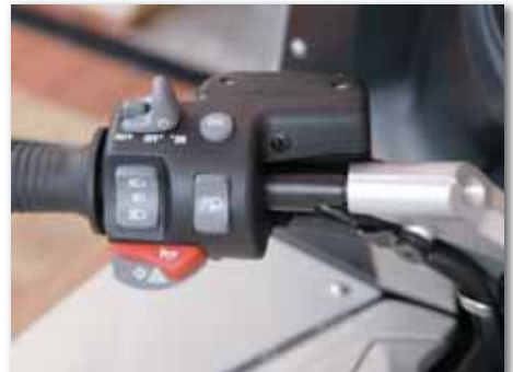
Easy access to controls with push-button electronic suspension adjustment, screen adjustment and cruise control.
